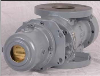
**Mechanical Standard Instrument Drive (STD-ID):** The standard instrument drive gas meter is a non-compensated instrument drive style meter that allows for installation of ancillary equipment. This equipment can include Volume Correctors, Pulsimatics or compensated indexes. This meter does not have a mechanical counter.
