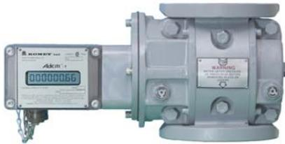
**Advanced Electronic Module Temperature Compensated (AdEM-T):** Electronic accessory unit with Pulse Output standard. Allows for very large turn-down, long battery life, live temperature compensation and fixed factor pressure compensation. Also displays volume and flow rate. Audit Trail is available.
