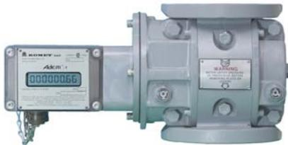
**Electronic Corrected Module 2-PTZ (ECM2-PTZ) Module:** Electronic accessory unit with Pulse Output standard. Allows for very large turn-down, long battery life, live temperature compensation, and live pressure compensation. Also displays volume and flow rate. Audit Trail is available.
