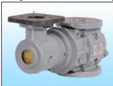
**Mechanical Temperature Compensated Counter (TC):** The temperature compensated digital counter style gas meter is for outdoor applications where the temperature of the flowing gas fluctuates widely (more than +/- 3°F or 1.5°C).
