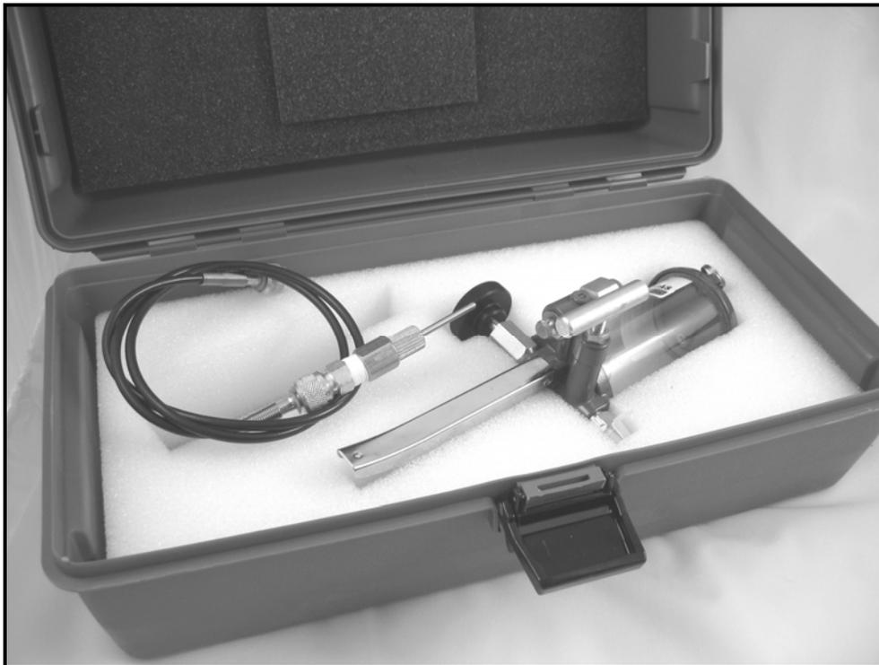
The Model R-2000 Oiler is a Hydraulic hand pump with pressure capacities from 0-2000 PSI. Internal parts are heavy duty, made from brass, aluminum, stainless steel, and Buna N. The transparent reservoir allows for quick check of fluid level. The bleed-off valve is capable of a slow bleed of pressure and fluid back to the reservoir. A built-in vernier fine tuning piston enables a precise control of pressure down to 100 PSI. *Optional:* Pressure Gauge and Model 510 (1/16") Probe
