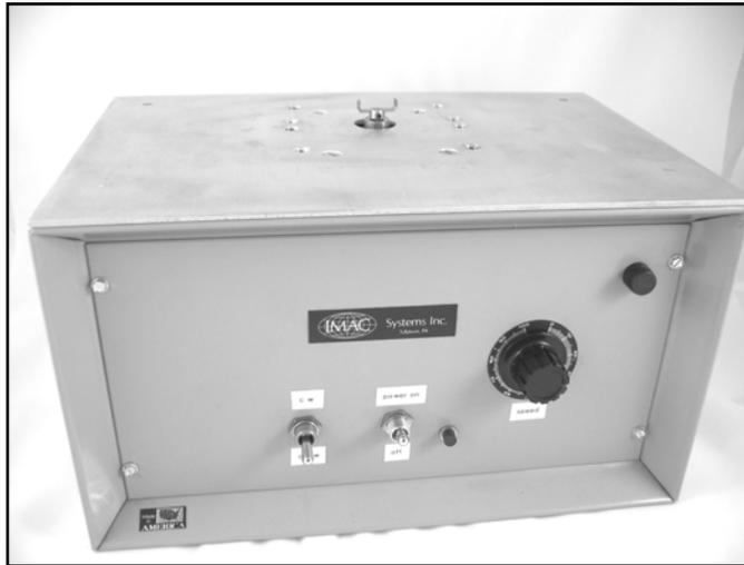
The IMAC I.T.F. (Instrument Test Fixture) is an easy way to emulate meter rotation for testing and calibrating instruments. The rotation speed and direction is set by the user. The test stand has multiple mounting patterns that allow for all common instruments. The required power supply is 120 volts a.c.
