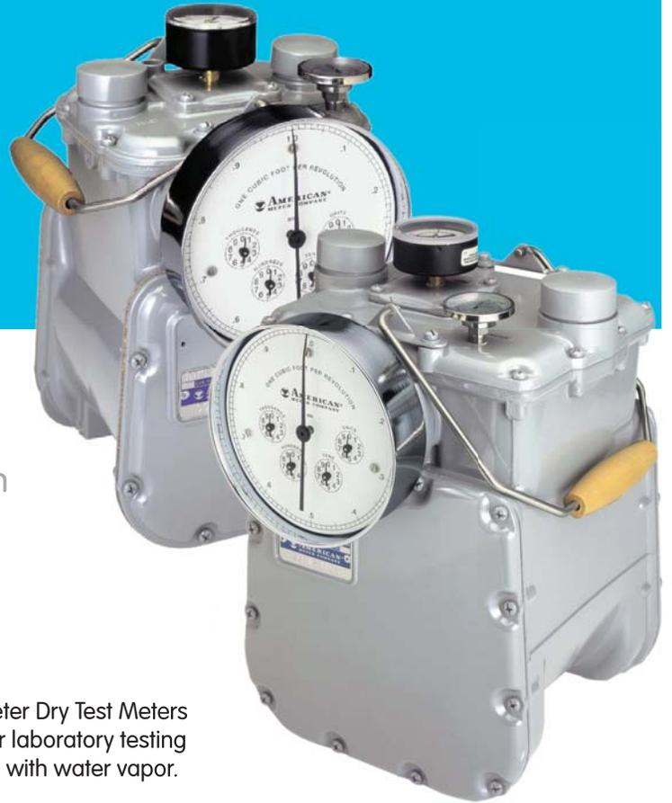
The Dry Test Meters are used for field or laboratory testing of various hydrocarbon or other non-corrosive gases to obtain highly accurate volume measurements.
