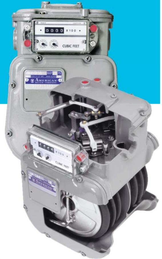
Special application, residential gas meter available in either 5 PSIG or 10 PSIG Maximum Allowable Operating Pressure with a badge rate of 250 cfh (.60 gravity gas) at 1/2-inch W.C. differential pressure.
