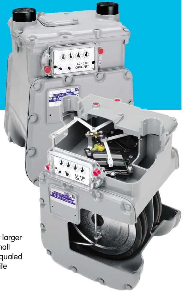
Designed to meter a variety of gases for large residential/commercial/small industrial applications at pressures up to 25 PSIG and flow rates to 630 SCFH at 1/2" W.C. differential pressure
