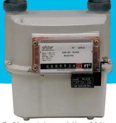
The G4 gas meter is a remarkably small, lightweight meter ideally suited to residential submetering applications. Despite its small size, the G4 meter is incredibly accurate and reliable when measuring either natural or LP gas. The G4 is classified as a 200 cubic foot per hour (cfh), non-temperature compensated gas meter with cyclometer register.
