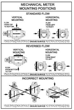
\*To install in meter in a reversed flow configuration, flow configuration must be switched by factory\*
