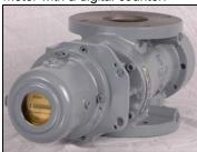
**Mechanical Standard Instrument Drive (STD-ID):** The standard instrument drive gas meter is a non-compensated instrument drive style meter that allows for installation of ancillary equipment. This equipment can include Volume Correctors, Pulsimatics or compensated indexes. This meter does not have a mechanical counter.
