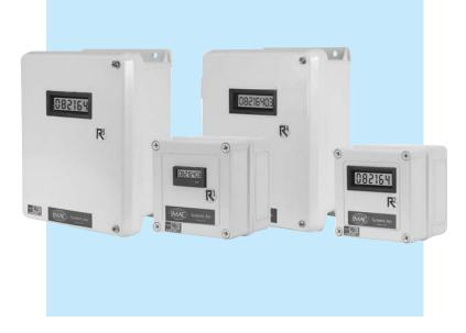
\*NEMA 4 enclosures are intended for indoor and outdoor use. They provide protection against windblown dust, rain, splashing and hose directed water. The fiberglass reinforced polyester construction allows the product line to be nonconductive, lightweight and impact resistant.
