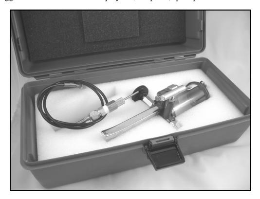
The Model R-2000 Oiler is a Hydraulic hand pump with pressure capacities from 0-2000 PSI. Internal parts are heavy duty, made from brass, aluminum, stainless steel, and Buna N. The transparent reservoir allows for quick check of fluid level. The bleed-off valve is capable of a slow bleed of pressure and fluid back to the reservoir. A built-in vernier fine tuning piston enables a precise control of pressure down to 100 PSI. *Optional*: Pressure Gauge and Model 510 (1/16") Probe
