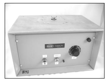
The IMAC I.T.F. (Instrument Test Fixture) is an easy way to emulate meter rotation for testing and calibrating instruments. The rotation speed and direction is set by the user. The test stand has multiple mounting patterns that allow for all common instruments. The required power supply is 120 volts a.c.
